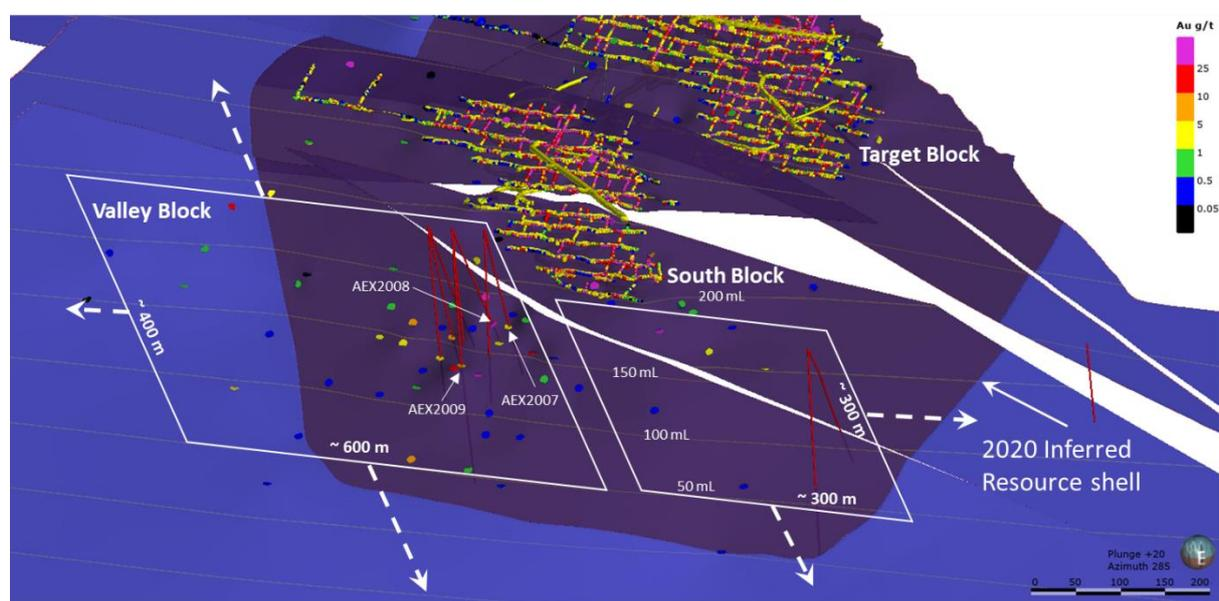
**Figure 1** Preliminary outline of the “Valley Block”. 2020 drillhole traces shown in red.
